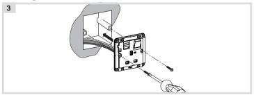
After wiring, fix the device with the two screws attached into the wall box (3).
