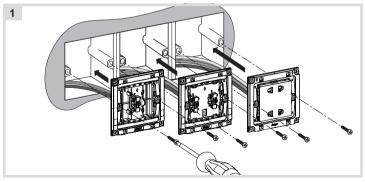
After wiring, fix the devices with the screws into the wall boxes (1).
