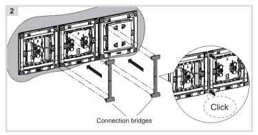
Align one bridge per connection and clip the bridges one after the other in the supporting plates of the devices (2).
