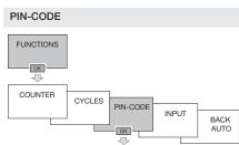
The menu PIN CODE allows you to lock the clock keyboard.
