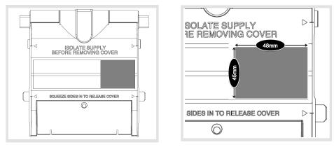
Mark the shroud ready for cutting out the aperture to allow the device to protrude through.
