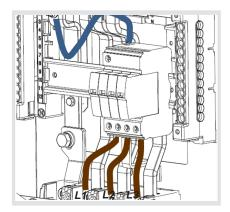
Connect the L1/L2/L3 cable lugs to the Incomer using the M8 Bolts provided making sure to use the flat washer and shake proof washer, torque to 13Nm
