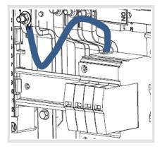
Connect Neutral cable to the neutral bar with the M5 hex Carp nut and torque to 5Nm
