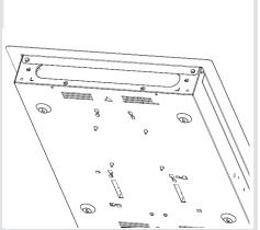
Secure the frame with the 2 Screws provided shown at the top and repeat the process at the bottom side of the board.
