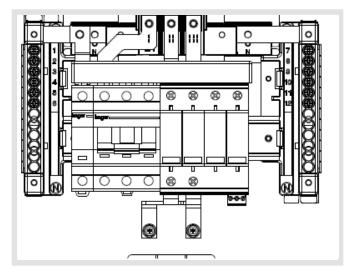
Place the copper earth component into the bottom two cage terminals and secure to 3.5Nm.
