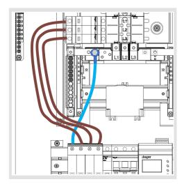
Clip the 4 module surge protection device to the dinrail next to the incomer. Fit the 3 KRN199 terminal block's to the first 3 phases on the left hand side of the busbar stack as shown above and torque to 3.5Nm.
