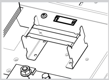
Fit the meter bracket onto the chassis using the fixings provided.
