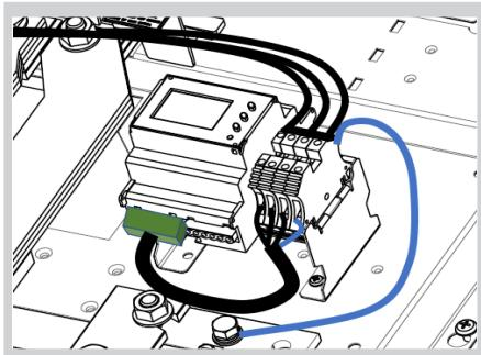
Remove the busbar shroud and fit Line & Neutral cables to the positions as shown above. Tighten to the required torque stated in the panelboard instructions.
