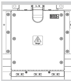
Fit the shrouds with the fixings provided.
