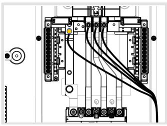
Finally connect the phase cables and neutral to the positions pictured above L1 - L2 - L3 & Neutral with the carp nuts provided and torque to 5Nm.
