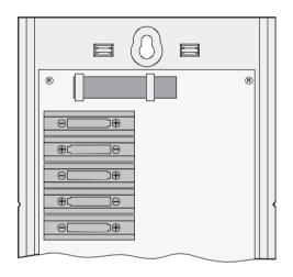
Fig. 1.c: Battery compartment inside the radio control unit
