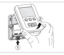
2. Open the flap with the help of a screwdriver and attach the wall-mounted base using the screws. 3. Next, pass the electrical cables into the holes intended for this purpose.
