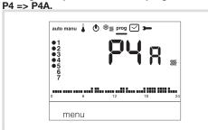
If the anticipation function (1H, 2H or 3H) ) in the Installer parameters PA:9 has been confirmed, P4R is displayed in place of P4.
