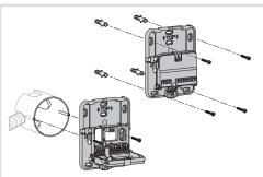
For optimum quality temperature regulation, seal the flush-mounted casing or the electrical duct. Separate the product from the wall-mounted base, by pushing on the button located under the base.
