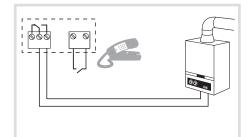
Connection of the thermostat to the thermostat input of a reversible or irreversible heat pump (HP)
