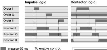
close contact 312 with Impulse maintened. For contactor logic bridge contact 316 with 317.
