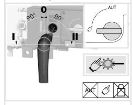
7D. Padlocking mode (Standard: in position O) Foreseen for max. 3 padlocks Ø 4-8mm
