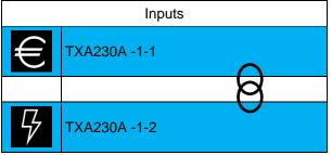
For the configuration tool to start the automatic link procedure there should only be one TXA230A master output module in the installation and no more than one TXA230B slave output module. The number of WKT660B input modules is unlimited.
