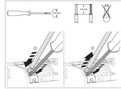
Fig 2: Installation/removal with plug-in terminals
