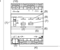
Figure 1 : Device overview (1) Slide switch auto/min/max/ (min/max
