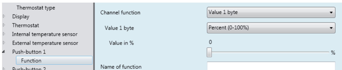
Figure 40: Function value transmitter 1 byte/2 byte
