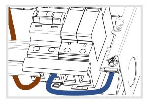
Push the busbar firmly against the Surge protection device making sure the cables below are secure secure and torque back to 3.6Nm.
