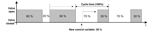
Before receipt of the new manipulated variable (30 %) the old setpoint (80 %) was active. The new manipulated variable is received during the closing phase of the valve. At this point in time the actuator recognises that it is still possible to cut short the closing phase so that it corresponds to the new manipulated variable (30 %). The cycle time remains unchanged, the starting time of the period is nevertheless automatically delayed.
