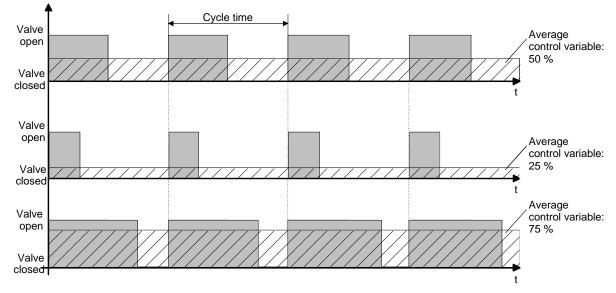
Based on the parameter "Mode of operation of valve / valve drive combination" for each output, the respective output is energised or not energised depending on the valve setting to be achieved. If the drive is "Current-free open", the duty cycle is automatically inverted. There is therefore no undesirable shift in the average based on the type of valve used.
