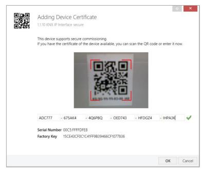
Figure 2 – Adding Device Certificate
