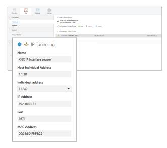
Figure 9 – IP Tunneling
