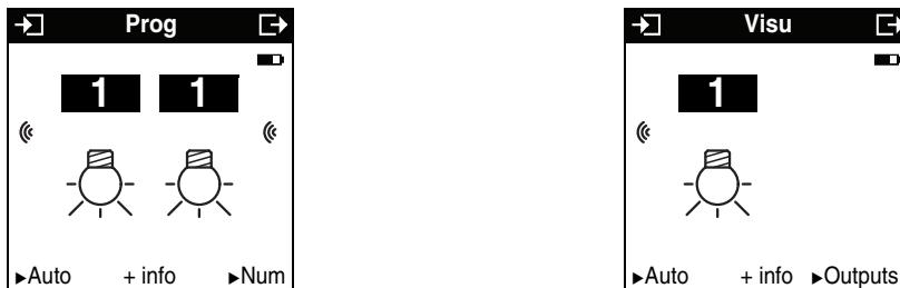
The +Info mode allows the status indication to be linked from an output to a viewing product: Area controller, LED output, etc. The status indication sends the current status over the network each time the status changes.
