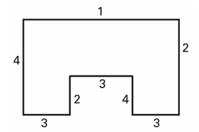
Even in buildings with a U-shaped layout, only 4 facades have to be controlled differently, as several have the same alignment.
