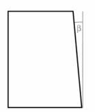
If a facade surface is not oriented horizontally, this must be taken into account. A forward inclination of the facade is counted as a positive angle; a backwards inclination (as in the picture) as a negative angle. This also allows a sunshade of a window built into a sloping roof surface to be controlled according to the current position of the sun.
