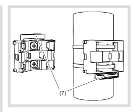
Figure 5: Wall fixing (left) or mast fixing (right) (7) crescent-shaped ba
