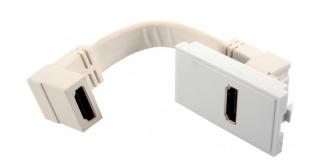
The HDMI module outlet comes complete with HDMI Type A high speed outlet (female) fitted into a 25mm x 50mm Euromodule plate with a 125mm flat fly lead with a right angled HDMI type A (female) outlet.
