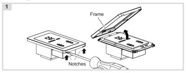
Carefully loosen the frame on the notches with a flat-blade screwdriver. Lift up and remove the frame (1).
