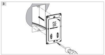
After wiring, fix the device with the two screws attached into the wall box (3).
