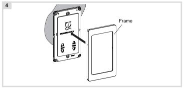
■ Snap the frame onto the device (4).
