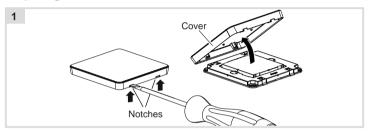
Carefully loosen the cover on the notches with a flat-blade screwdriver. Lift up and remove the cover (1).
