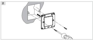
Fix the device with the two screws attached into the wall box (2).
