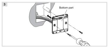
After wiring, fix the bottom part with the two screws attached into the wall box (3).
