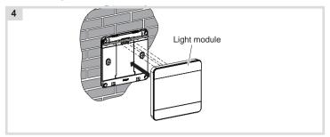
■ Place the light module in the correct position and snap it onto the bottom part (4).
