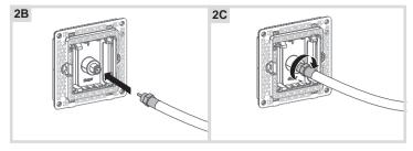
Connect and screw the assembled line to the F-jack on the rear of the TV outlet (2B/2C).
