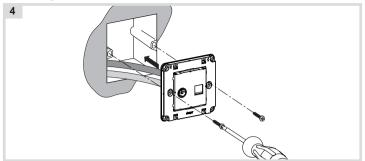
■ After wiring, fix the device with the two screws attached into the wall box (4).
