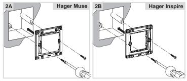
Fix the device with the two screws attached into the wall box (2A/2B).
