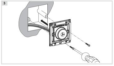
After wiring, fix the device with the two screws attached into the wall box (3).
