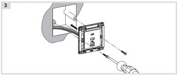
■ After wiring, fix the device with the two screws attached into the wall box (3).
