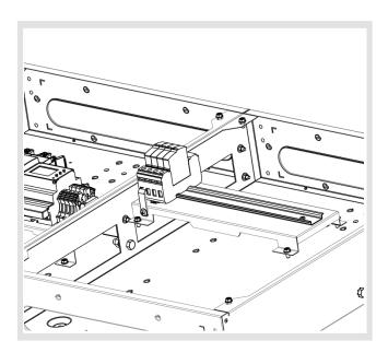
Screw the surge protection sub-assembly on the right hand side of the enclosure as shown using the 4 off Hex head High Torque screw to the chassis at 5Nm
