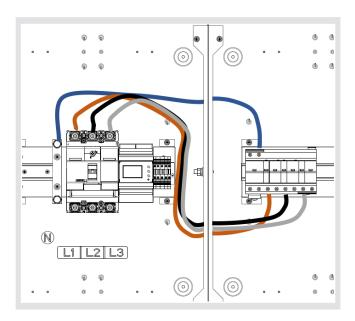
Connect the L1/L2/L3 cable lugs to the Incomer using the existing incomer bolts provided, torque to 13Nm and connect the Neutral cable to the neutral bar to the left of the MCCB, then terminate into the relevent terminals on the SPD
