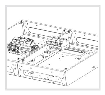
Screw the surge protection sub-assembly on the right hand side of the enclosure as shown using the 4 off Hex head High Torque screw to the chassis at 5Nm
