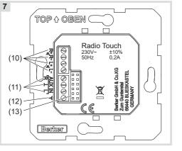
Connections on the radio insert (Figure 7) for: (10) Loudspeaker (L, R)
