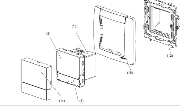
Figure 19: Assembly of the device
