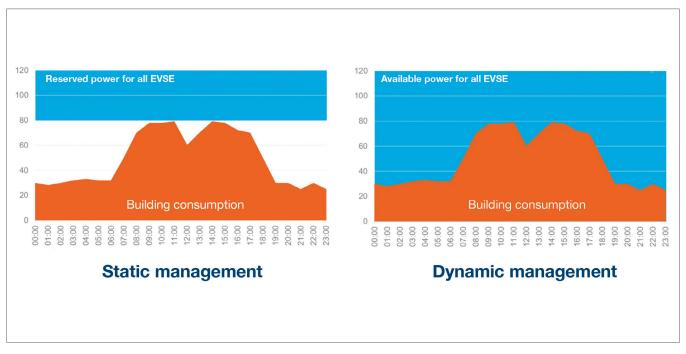
For buildings with multiple charging points, the Local Load Manager (LLM) makes it possible to adjust the power used to charge electric vehicles based on the total power consumption of the building. In the event of excessive consumption, corresponding protective mechanisms are triggered, avoiding a building-wide power failure. Using dynamic management, the available energy can be used to charge electric vehicles in full, without resulting in power failures.
