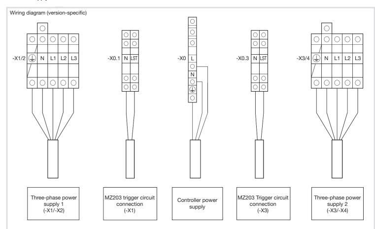
Power terminal block (230V/32A) for rigid cable of max. 10 mm<sup>2</sup>.
