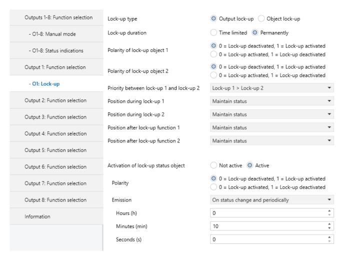
The Lock-up function is used to lock the output in a predefined state.
