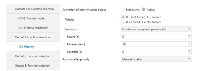
The Priority is used to force the output into a predefined state.
