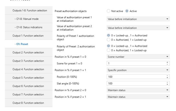
The Preset function is used to switch an output into various predefined states. The Preset function is activated via an object in 1-bit format.
