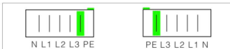
Installation position: Housing in flat position, conductor upright position
