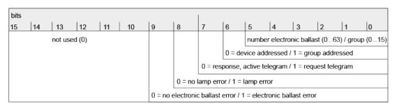
Figure 15: Telegram structure, 2-byte error status
