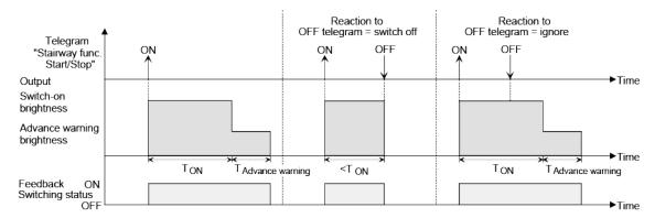
Figure 51: Switch-off behaviour of the staircase function without soft functions
