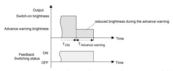
Figure 53: The pre-warning function of the staircase function without soft OFF function
