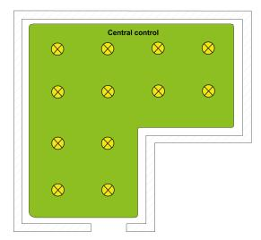
Figure 4: Example of a master control (broadcast) - Only one group
