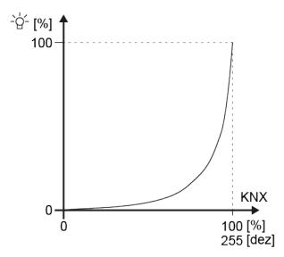
Figure 21: Logarithmic dimming characteristic curve at the output of an operating device
