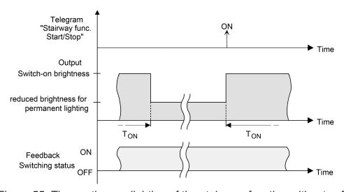
Figure 55: The continuous lighting of the staircase function without soft functions
