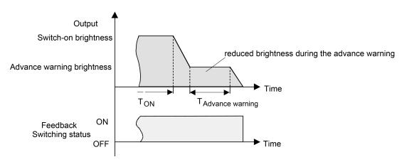
Figure 54: The pre-warning function of the staircase function with soft OFF function (as an example with minimum brightness = 0%)
