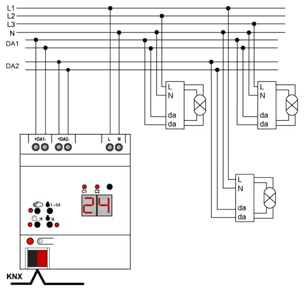
Figure 2: DALI gateway connection example, 2fold
