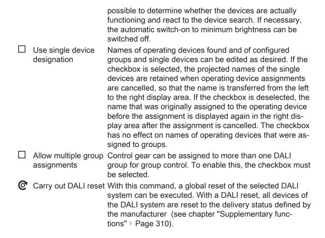
In the display area for found devices (H), a separate context menu is available for each operating device, via which DALI online functions can be called up with which selected devices can be identified in the DALI system. These operating devices can be made to switch-on, switch-off and flash (cyclical ON and OFF). The device context menu is called up when one or more devices are selected in the display area and then the right mouse button is clicked.
