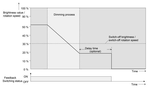
Figure 48: Dimming and switching behaviour of the automatic switch-off function
