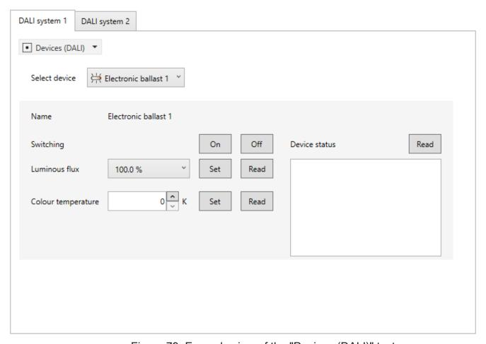
Figure 79: Example view of the "Devices (DALI)" test
