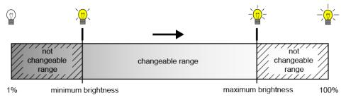
Figure 41: Brightness sequence direction "brighter"
