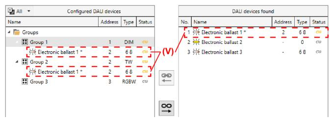
Figure 71: Example for multiple group assignment of a DALI operating device
