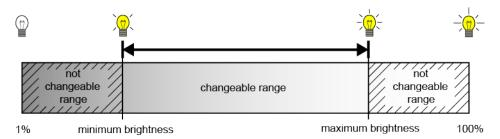
Figure 40: Brightness sequence during automatic brightness sequence
