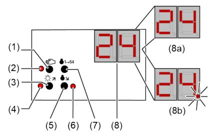
Figure 10: DALI gateway control panel, 1-gang
