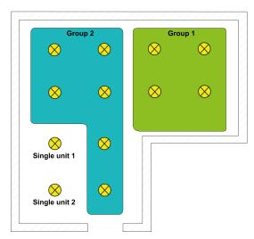
Figure 7: Example of group and single device control
