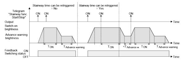
Figure 50: Switch-on behaviour of the staircase function with soft functions (as an example with minimum brightness = 0 %)
