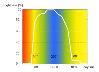
Figure 44: Exemplary daytime colour sequence with colour and brightness adjustment
