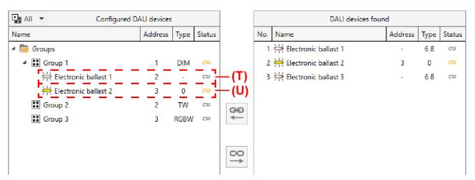
Figure 69: Example of virtual devices of a projected DALI group
