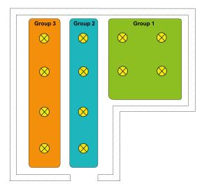
Figure 5: Example of group control with three groups - all lights with group address-ing
