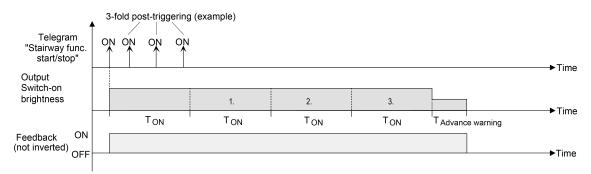
Figure 57: Time extension of the staircase function
