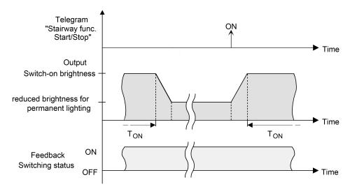
Figure 56: The continuous lighting of the staircase function with soft OFF functions
