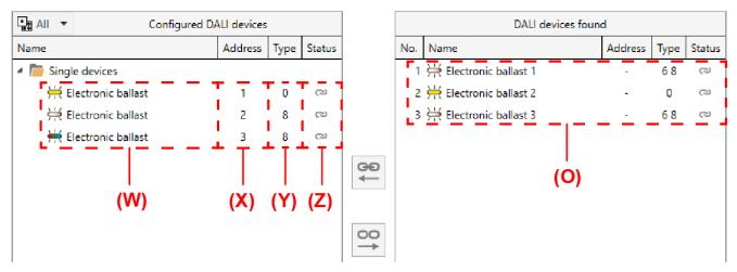
Figure 72: Example of projected DALI single devices in the left display area
