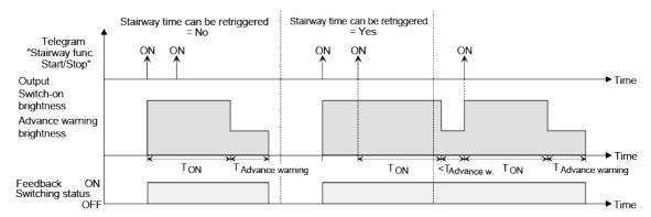
Figure 49: Switch-on behaviour of the staircase function without soft functions
