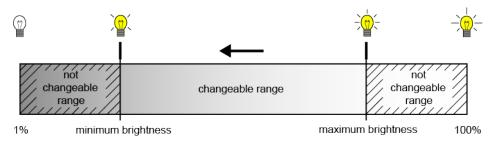
Figure 42: Brightness sequence direction "darker"
