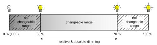
Figure 18: Example of a dimmable brightness range
