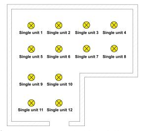
Figure 8: Example of single device control - All the DALI operating devices can be controlled individually
