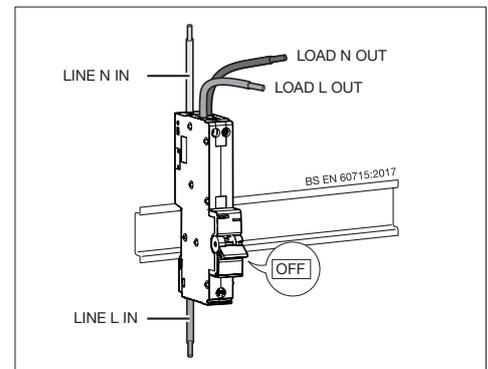
Fig 4: Connect the MCB-AFDD
