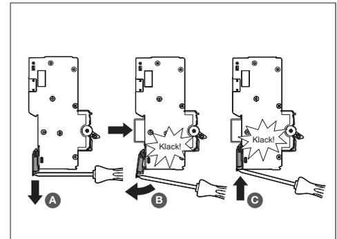
Fig 3: Mounting the MCB-AFDD
