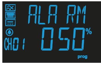
Fig. 37: Pre-alarm trip current
