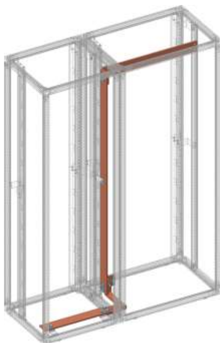
Main PE traversal front the front, bottom, to rear top with the option of an outgoing PE at the bottom
