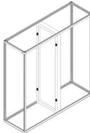
Position of internal connections of enclosures mounted in a row, at least 4 connections
