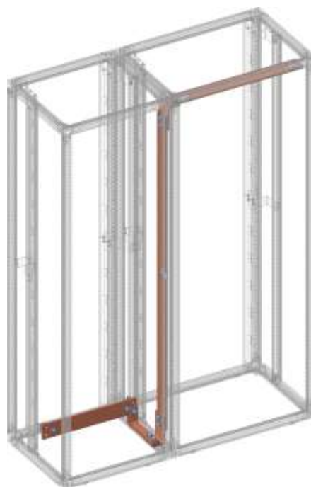
Main PE traversal from the rear, bottom, to front top
