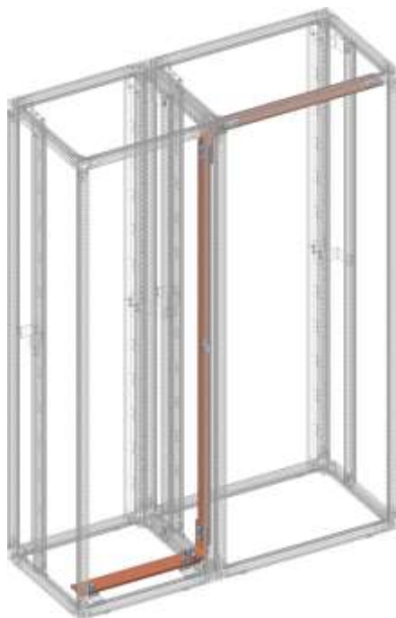
Main PE traversal from the front, bottom, to front top
