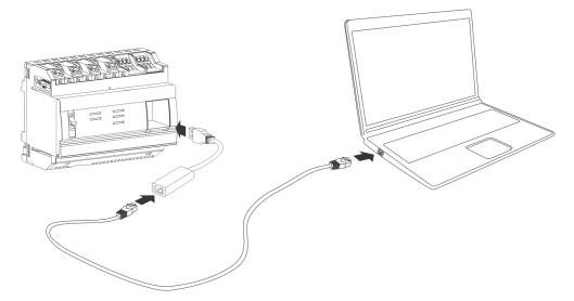
The HTG457H is a USB to RJ45 Ethernet interface, especially suitable for local connection with the energy monitoring server using a computer. The HTG457H allows direct connection on the front panel, avoiding any removing of a cover.
