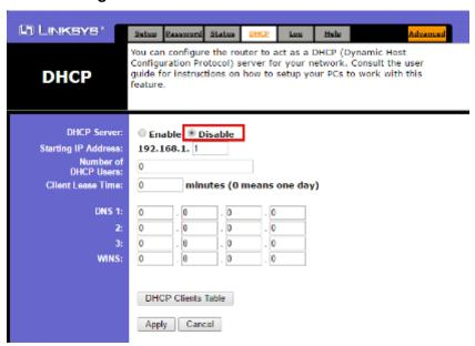
Hager recommends to use a static configuration of the energy monitoring server (**Method**: *Manual*). In consequence the LAN gateway (router or firewall) must use the same configuration (i. e. DHCP Server has to be disabled).
