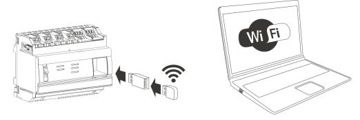
The HTG460H WLAN dongle is a USB to Wi-Fi interface, especially suitable for the connection without wire with the HTG411H/HTG411L. It allows direct connection on the front panel. This is the easiest mean to connect a computer or a tablet.
