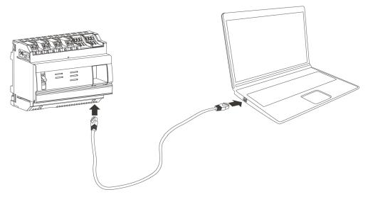
The setup mode is activated. The energy monitoring server acts as the DHCP server.
