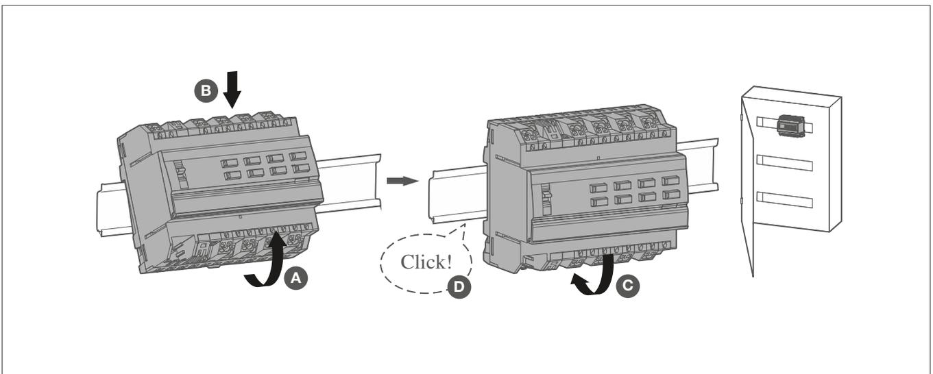
Fig. 4: Installing the device on the DIN rail
