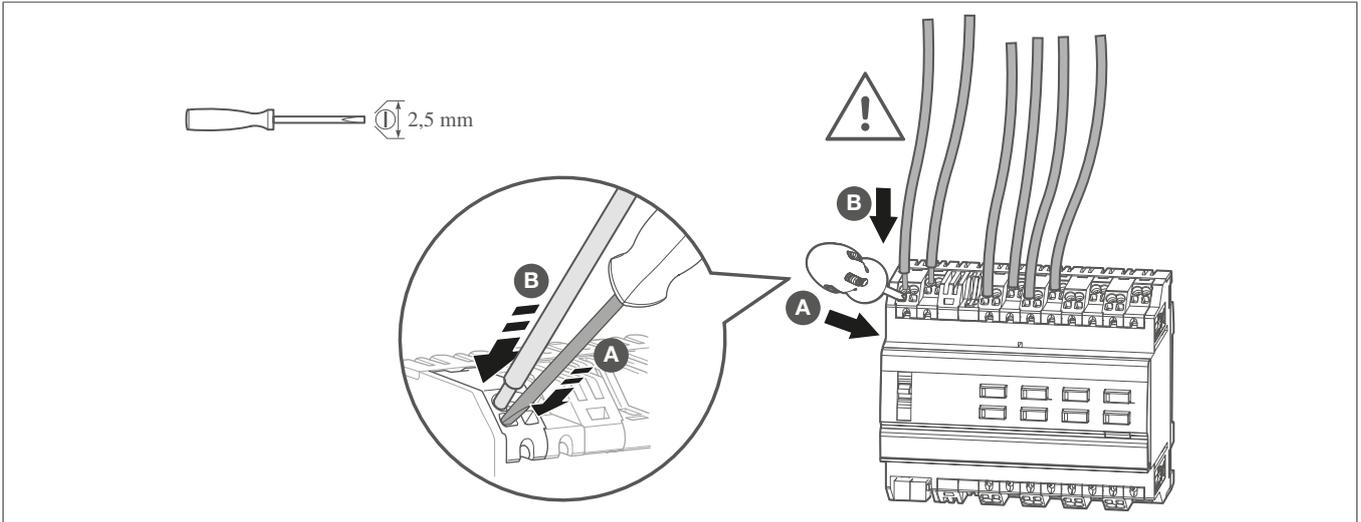
Fig. 5: Connecting the device
