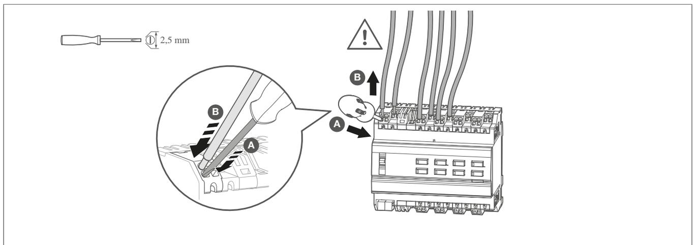
Fig. 13: Disconnecting the connection cables
