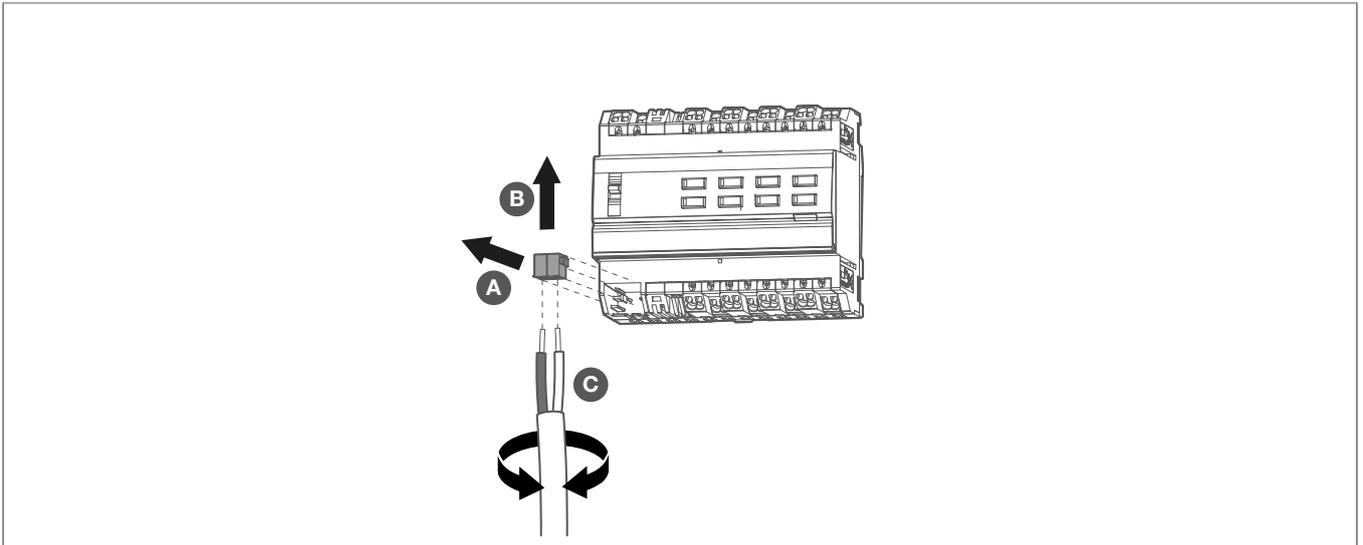
Fig. 14: Removing the bus connection terminal
