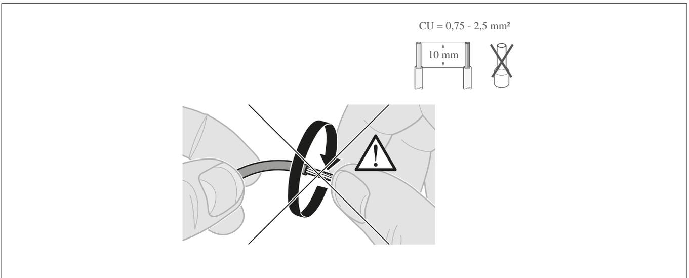
Fig. 6: Stripping length and cable cross-section
