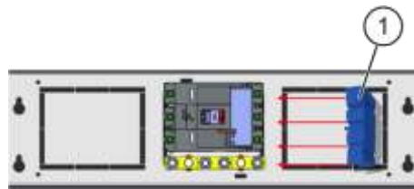
1 Disconnector link (Schematic representation)
