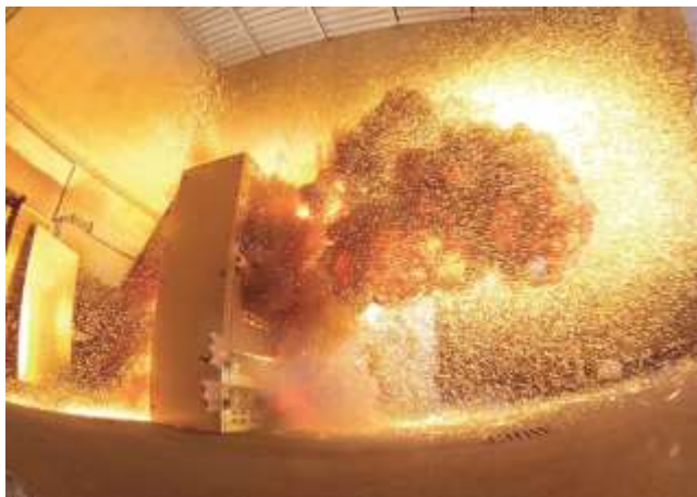
Provoked arc fault if there is no arc fault protection
