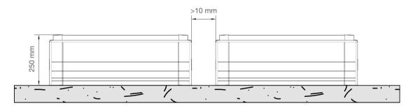
On-ground socles must be mounted on a suitable flat foundation. The gap between socle and foundation should be less than 1 mm to ensure the protection against ingress of solid objects of IP4X in this area. The following table shows the recommended frame conditions.
