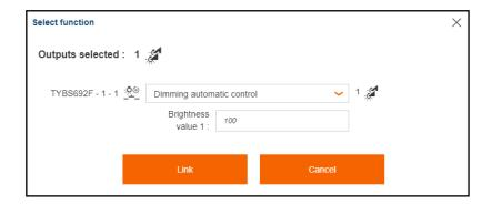
Dimmer switch automatic control: allows varying the light with two defined brightness values according to the opening and closing input contact using automatic control.
