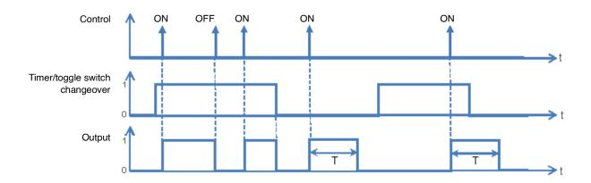
Communication objects: 6 - Output 1 - Timer/toggle switch changeover (1 bit - 1.001 DPT\_Switch)
