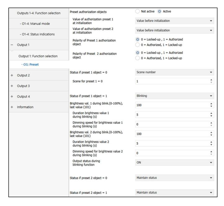
The Preset function is used to switch an output into various predefined states. The Preset function is activated via an object in 1-bit format.
