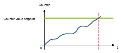
The counter starts to count up from the value 0. As soon as the counter setpoint (**Hours counter setpoint** object) is reached, the **Hours counter setpoint reached** object is set to 1 and sent to the bus.
