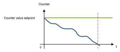
The counter starts to count down from the operating hours counter setpoint (**Hours counter setpoint** object). As soon as the counter reaches 0, the **Hours counter setpoint reached** is set to 1 and sent to the bus.
