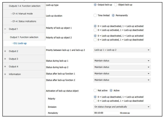
The Lock-up function is used to lock the output in a predefined state.
