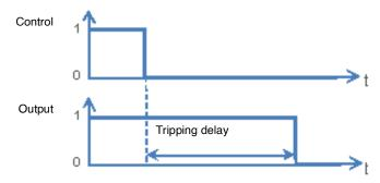
**Switching and tripping delay**: Allows the configuration of a delay between the switch-on command and the switching of the output contact, as well as between the switch-off command and the switching of the output contact.
