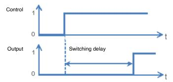
**Tripping delay**: Allows the configuration of a delay between the switch-off command and the switching of the output contact.
