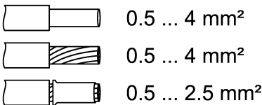
Figure 4: Clampable conductor cross-sections Load outputs and power supply
